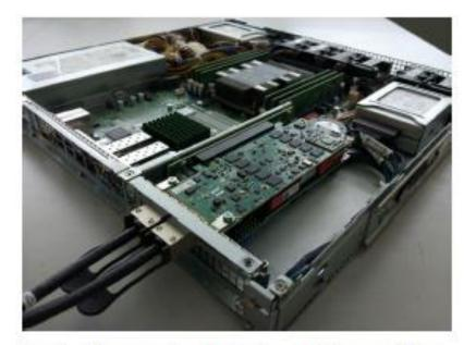
Fig. 2 Active network probe implemented in a small factor server. FPGA is placed in the bottom corner, with both QSFP28 interfaces connected. Management interfaces are on the left. Optical paths created dynamically by SDN infrastructure can be checked before they are put in operation
