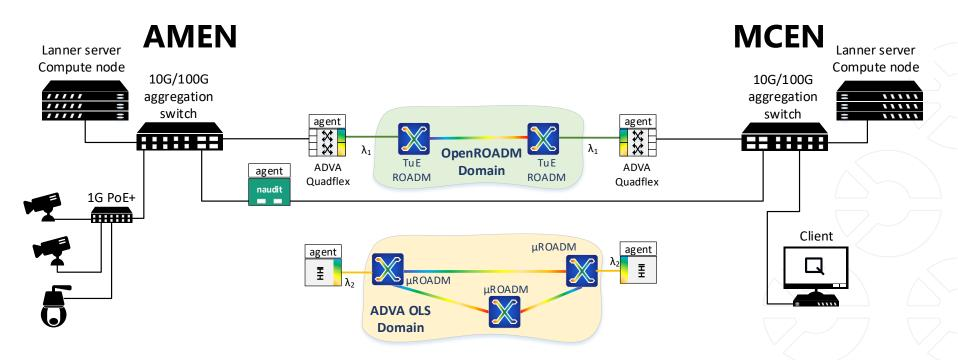
Compute nodes and cameras are connected via switches Real-time traffic either through OpenROADM or ADVA OLS domain
