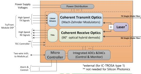
TIA: Transimpedance amplifier TEC: Thermoelectric cooler
