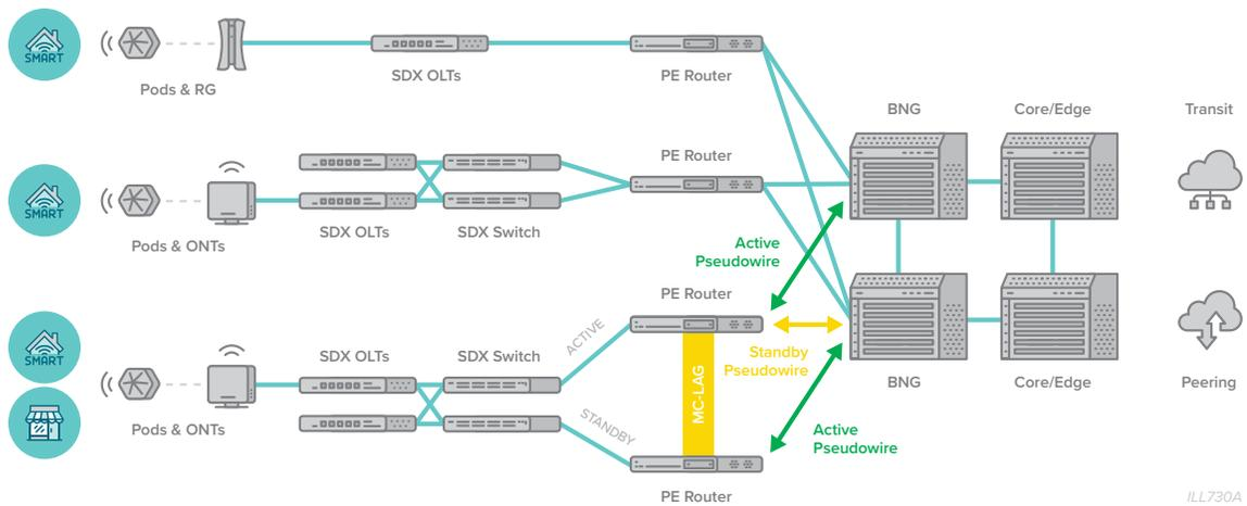
An alternative to MC-LAG, is to an EVPN-ESI which would allow an active/active connection downstream to the PON network. The connections to the BNG could then be built using an EVPN-VPWS service to provide an active / active connection to the BNG.
