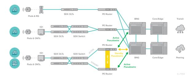
An alternative to MC-LAG, is to an EVPN-ESI which would allow an active/active connection downstream to the PON network. The connections to the BNG could then be built using an EVPN-VPSW service to provide an active / active connection to the BNG.
