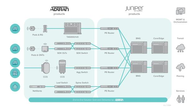
The BNG sits at the backbone or physical core of a network. It is a high-capacity device that serves as the gateway to the Wide Area Network (WAN) or the internet. A BNG architecture is designed to do the following:
