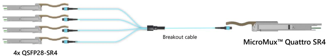
MicroMux™ Quattro converts a 400GbE port into four 100GbE ports with zero footprint increase
