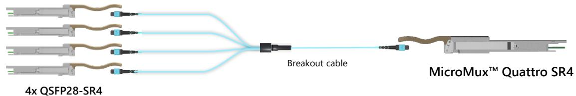
MicroMux™ Quattro converts a 400GbE port into four 100GbE ports with zero footprint increase
